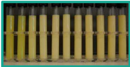
* Electrolyte scan with 10% colored MWF starting with DE Water (0 ppm) and increasing concentration of magnesium
